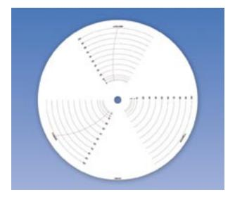
THIN-The thin Calibration Discs are made of a high quality Kodak<sup>®</sup> film.
